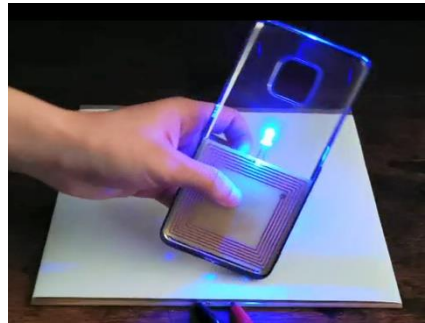
Fig. 3 Wireless Charging of a Mobile Phone
