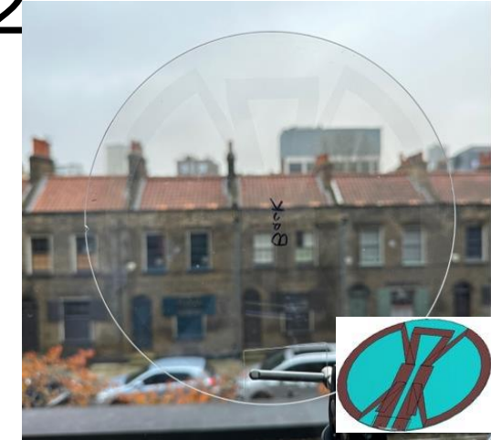
TV antenna patterned on Glass @400-800 MHz
