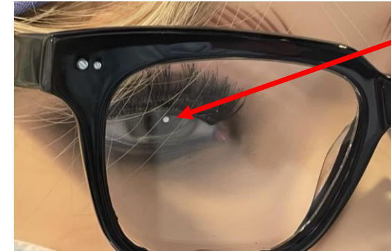
AR glasses with Transparent 5G antenna
