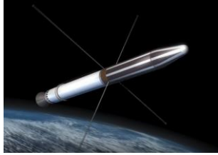
Explorer 1 (1958) Two Whip Antennas operating at 108 MHz. Discovered Van Allen Radiation Belt
