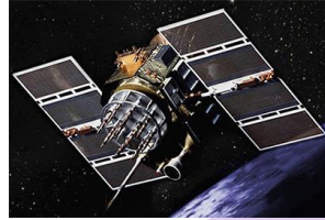
Navstar (1978) Dish and Patch Antennas at S and L Band for GPS
