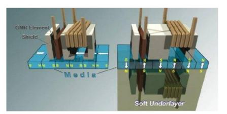
Perpendicular recording allows larger "write" magnetic fields to be used
